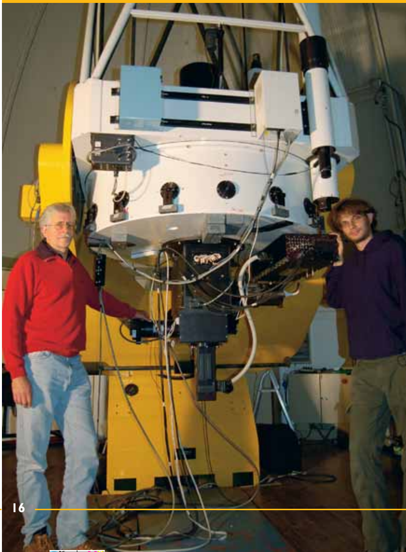
▼ Fig. 6: OPTIMA-Burst mounted on the 1.3m telescope
